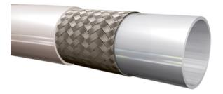
By integrating a metal- or plastic-based braiding into the tube wall, the mechanical properties can be significantly improved. For example, high torsional stiffness or even low bending radii can be achieved with thin wall thicknesses. The classic field of application for such tubes is flexible endoscopy.
