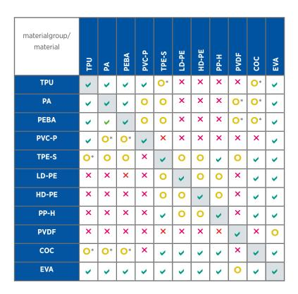
Co-extrusion of incompatible material types is possible through the use of modified polymers as well as through the introduction of adhesion promoting layers.
